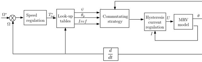
Fig. 7. Block diagram of the SRM drive with ATC.
