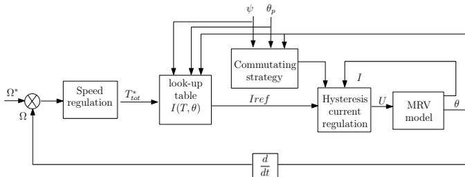
Fig. 3. Block diagram of the SRM drive with ITC.
