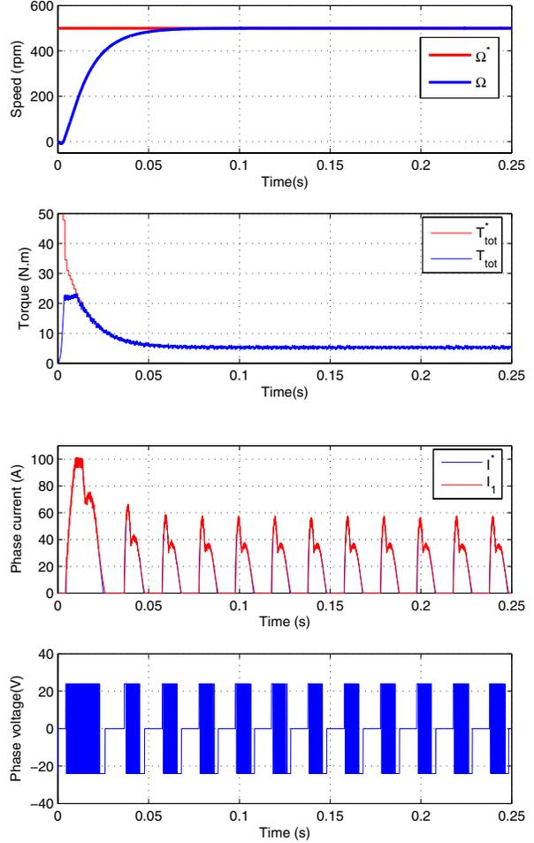
Fig. 4. Simulation results for instantaneous torque control.
