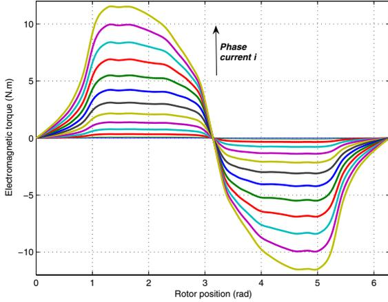
Fig. 1. Electromagnetic torque versus current and rotor position.
