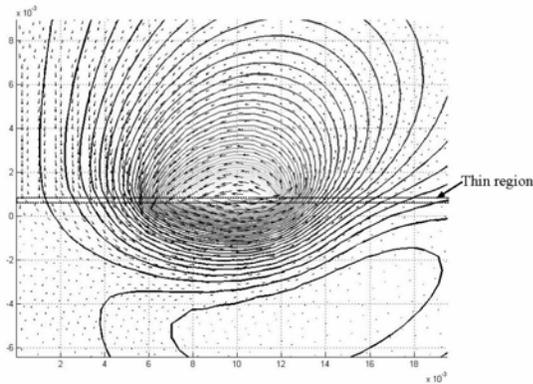
Fig. 2. Spatial distribution of the real part of magnetic flux density vectors and field lines obtained in the  $\mathbf{a}^*$  formulation.
