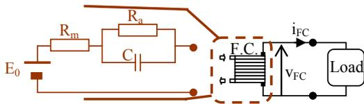
Fig. 1. Equivalent circuit representing the fuel cell
