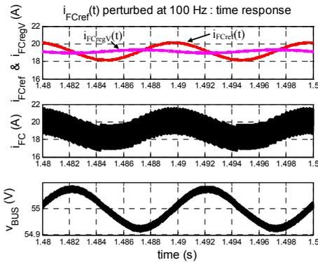
Fig. 6. AC perturbation superimposed to the voltage controller output (100 Hz)
