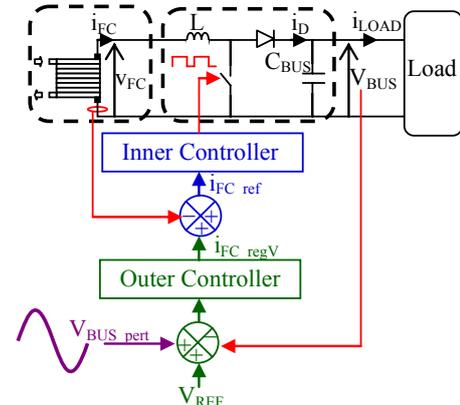
Fig. 8. AC perturbation by superposing an AC voltage
