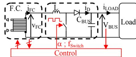
Fig. 2. schematic diagram of an integrated fuel cell system.
