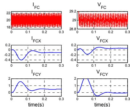
Fig. 13. Monitoring time response (AC perturbation at 100 Hz)
