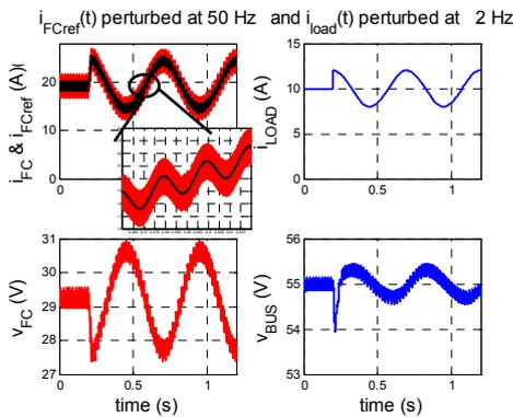
Fig. 11. AC perturbation superimposed to the voltage controller output (50 Hz) while a AC perturbation occurs at the load side (2 Hz)
