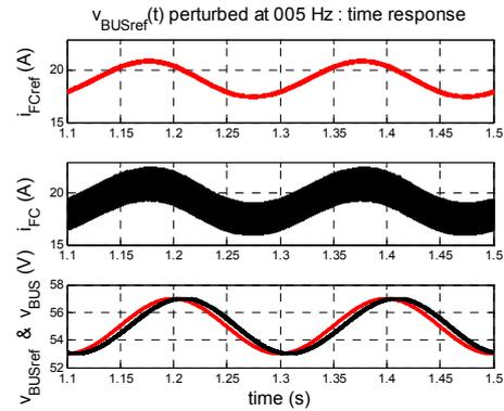
Fig. 9. AC perturbation superimposed to the constant reference of the voltage controller (5 Hz)
