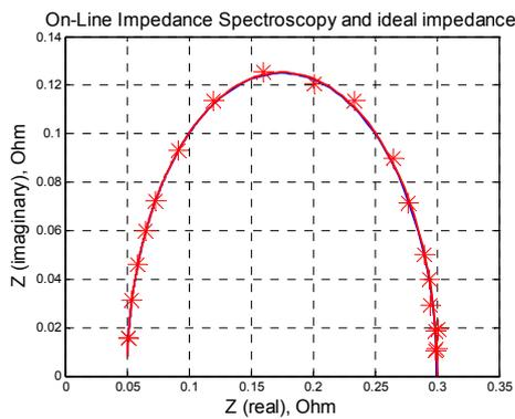
Fig. 14. Nyquist diagram (stars based on monitoring, line based on Randles structure)
