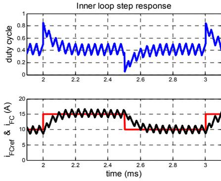
Fig. 3. Inner loop step response (DC chopper operating at  $F_{\text{Switch}} = 25$  kHz).
