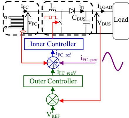
Fig. 5. AC perturbation by superposing an AC current
