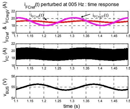
Fig. 7. AC perturbation superimposed to the voltage controller output (5 Hz)
