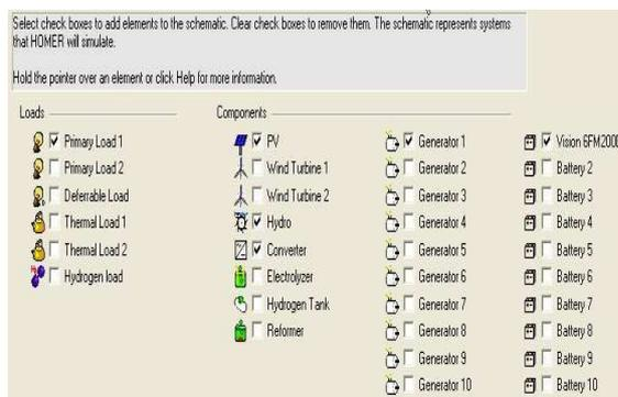
Fig. 1 HOMER available hybrid system components
