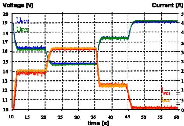
Fig. 15. Multi-stack power architectures. Experimental balance current tests performed on 2 PEMFC stacks for different load current steps.
