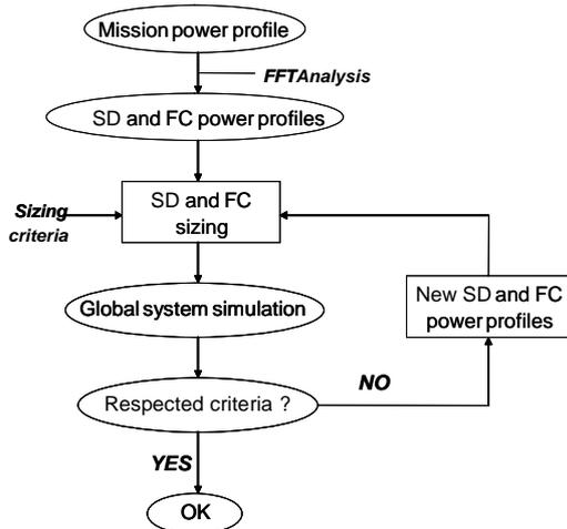
Fig. 6. Global sizing procedure of the hybridization between a fuel cell and a storage device.
