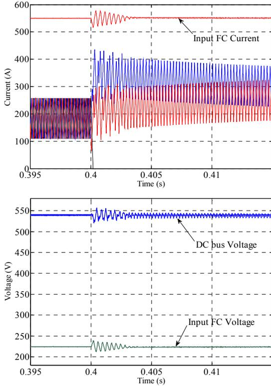
Fig. 18. Boost converter phase-leg out of work. Boost converter currents after fault detection (top) and DC bus and FC voltages during transient (bottom).
