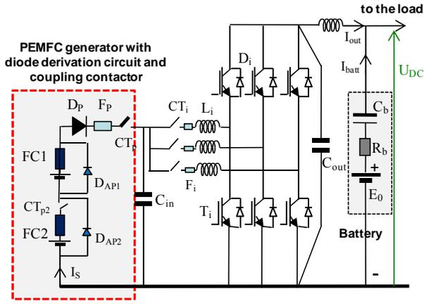
Fig. 16. Fault tolerant hybrid PEMFC/battery architecture for power transport application.
