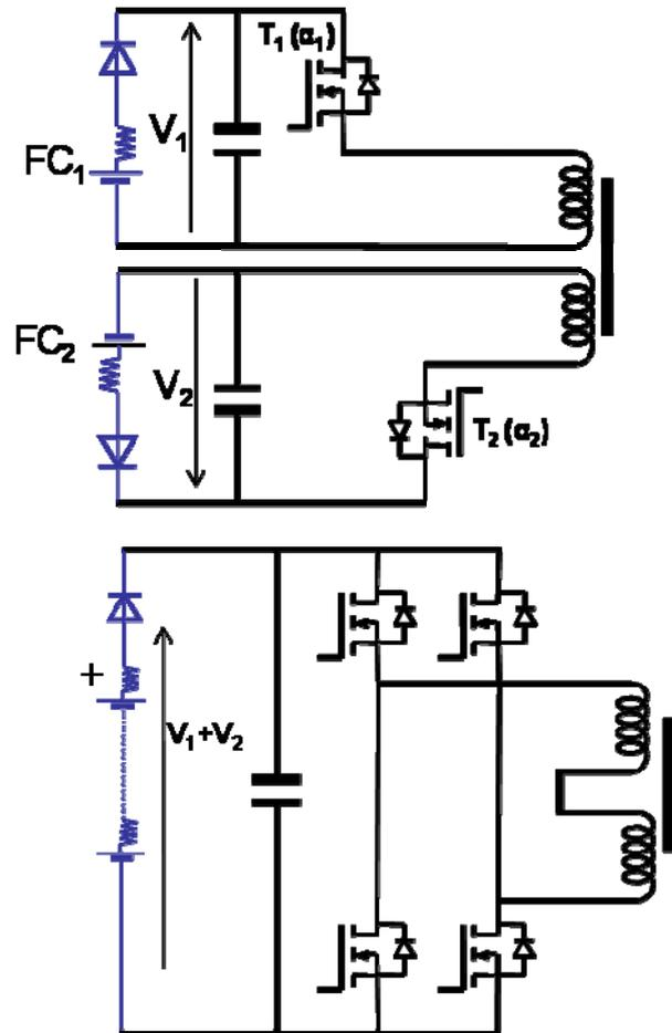
Fig. 13. Multi-stack power architectures, first stage converter topology, "pseudo-parallel" association (top), and series association (bottom).
