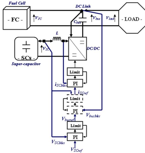
Fig. 10. Hybrid Power Source, FC and SC. Example of control strategy block diagram for a Direct Parallel Structure.
