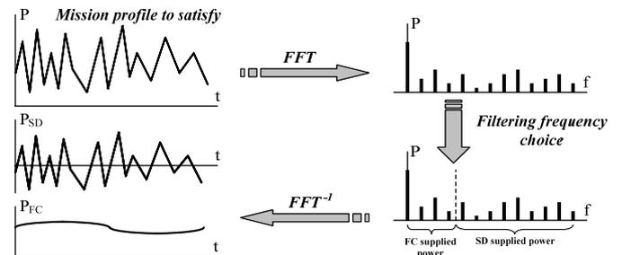
Fig. 5. Power sharing method between fuel cell and storage device.
