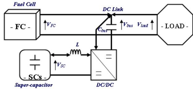
Fig 4. Direct Parallel Structure for hybrid power system associating FC and SC.
