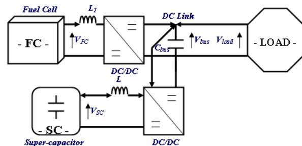
Fig. 1. Parallel structure for hybrid power system associating FC and SC.
