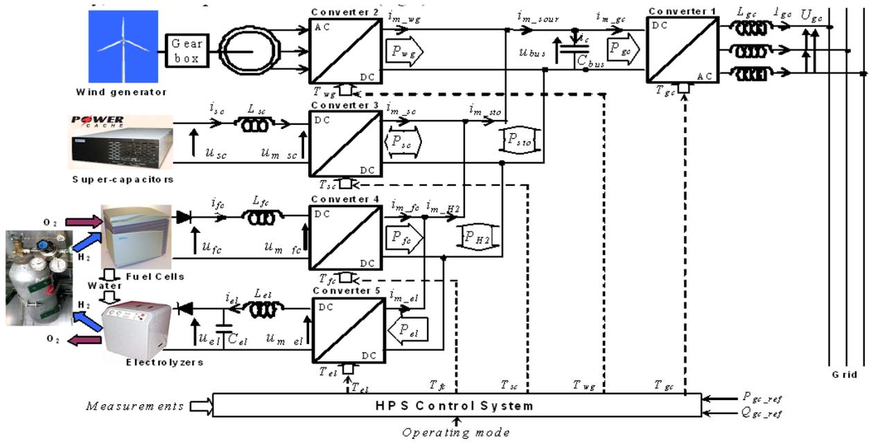
Fig. 19. Structure of the multi-source hybrid power system.
