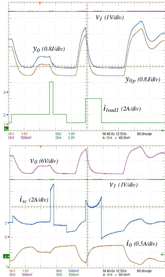
Fig. 12. Hybrid system with two independent loads, experimental results during load variations [27].
