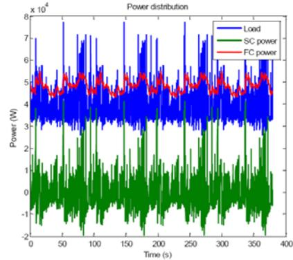
Fig. 7. Example of sizing results for direct coupling of a fuel cell and supercapacitors [16, 18].
