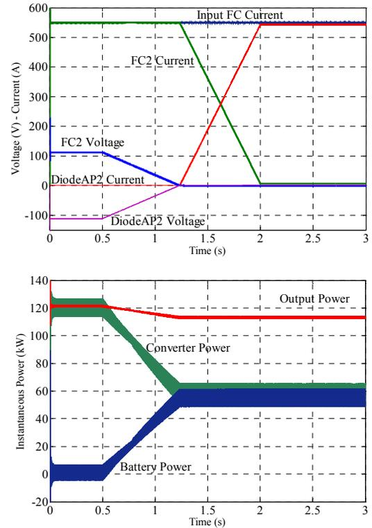
Fig. 17. FC2 stack out of work and power compensation (simulation results). Transient phase during fuel cell failure (top) and power compensation by the battery (bottom).
