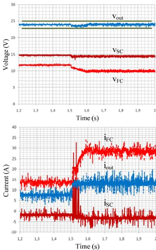
Fig. 3. Example of response to a load step [14].
