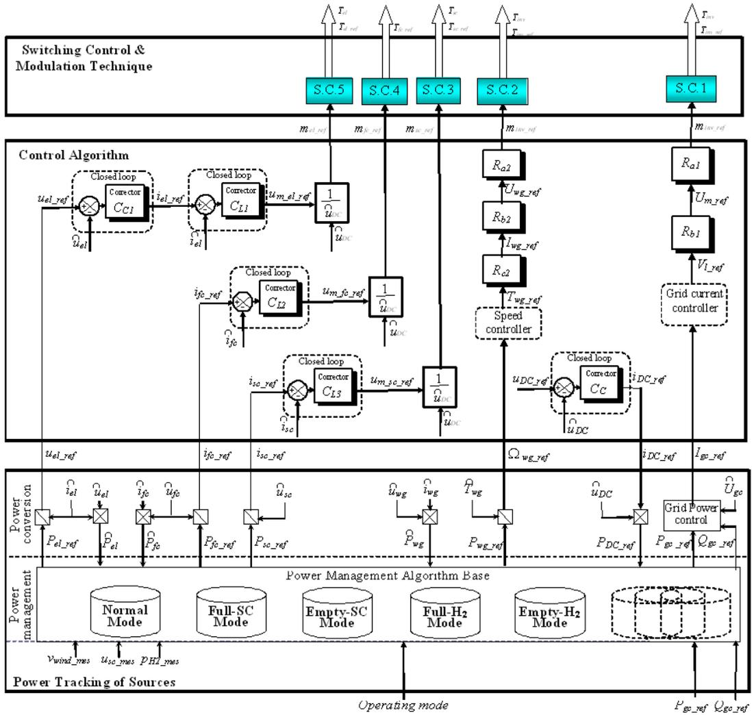
Fig. 20. Control system of the hybrid power system.
