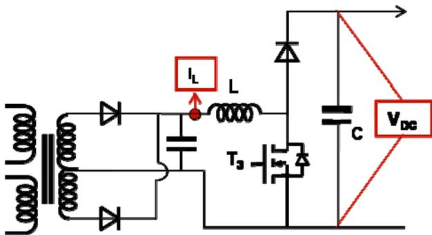
Fig. 14. Multi-stack power architectures, second stage adaptive booster.
