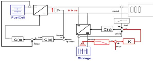
Fig. 9. Control strategy with the DC voltage imposed by the fuel cell converter.
