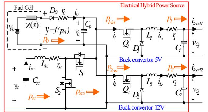
Fig. 11. Hybrid system with two independent loads [27].
