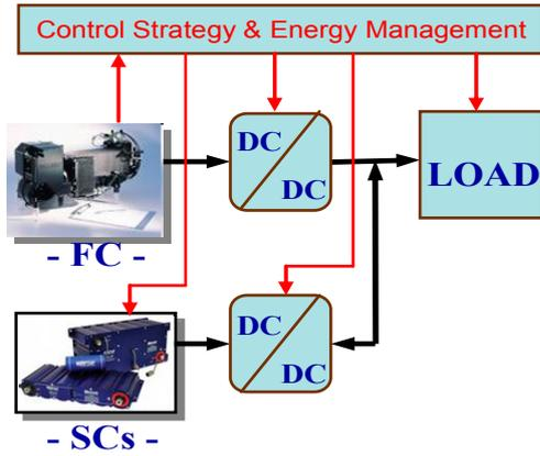
Fig. 1. Block diagram of a hybrid power system.
