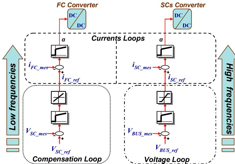
Fig. 4. Block diagram of control-command management strategy
