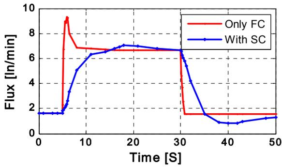
Fig. 8. Hydrogen mass flow consumption.
