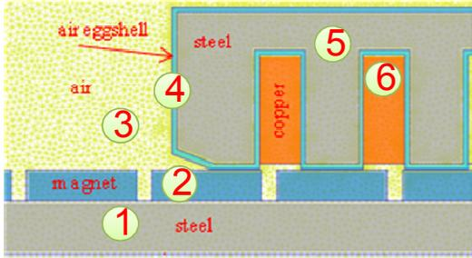
Fig.4. Geometry with mesh size of 0.3 mm [10].
