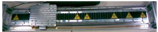
Fig. 1. Flat Ironcore PMSLM, LMD10-050 (ETEL).
