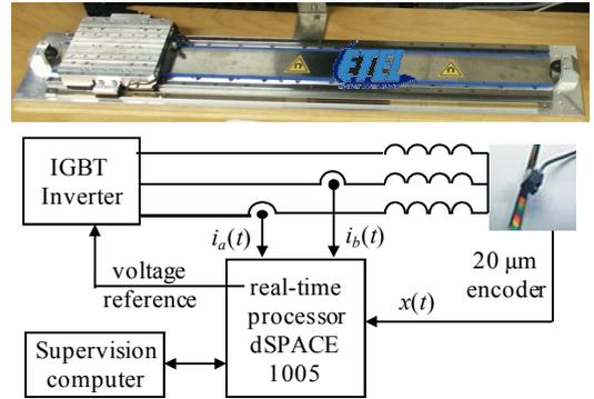
Fig.5. Experimental estimation of the force ripples.
