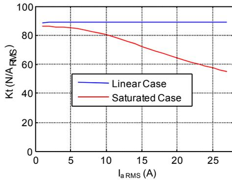
Fig.10. Impact of the saturation on Thrust Coefficient  $K_t$ .
