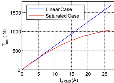
Fig.9. Impact of the saturation on Thrust generation.
