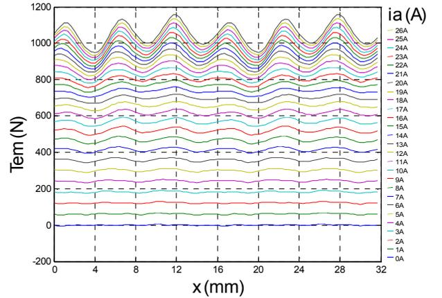
Fig.7. Thrust as a function of currents and magnets position.
