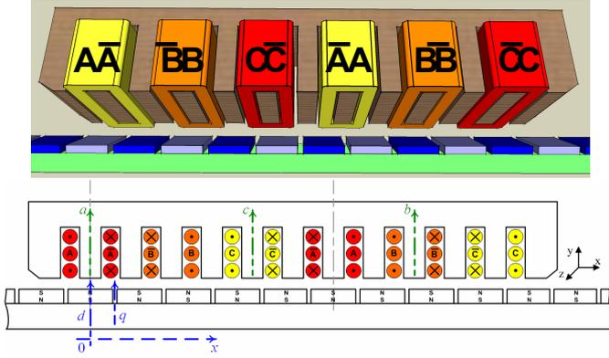
Fig. 2a. 3D view of a section of the whole PMLSM
