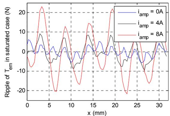
Fig.8. Influence of currents on ripple force of  $T_{em}$ .
