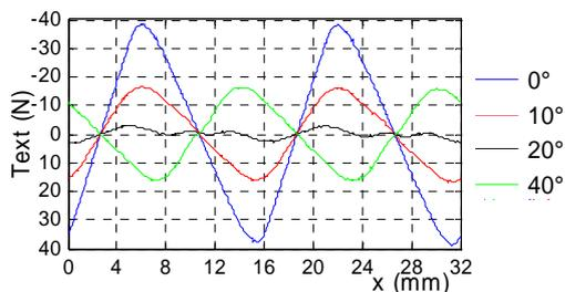
Fig. 18.  $T_{ext}$  using FEM with different angles of the extremities tooth
