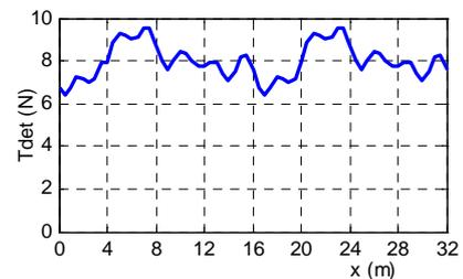
Fig. 1. Detent force with MST formulation
