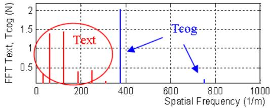
Fig. 17. FFT of the Detent force using the FEM
