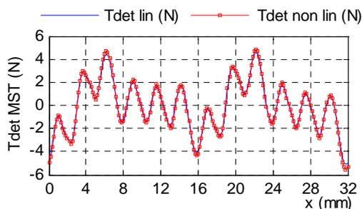
Fig. 8. No load force of a LMD10-050 (ETEL)
