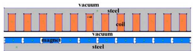
Fig. 11. Geometry for cogging force calculation<sup>(28)</sup>
