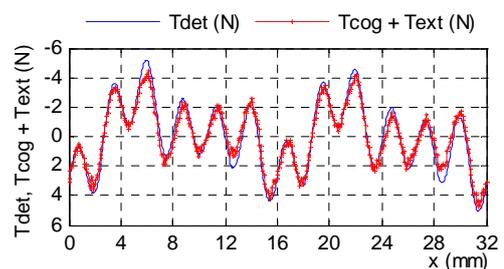
Fig. 16. Comparison between the sum of both forces and the total no-load force. (Linear case)
