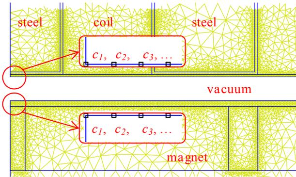
Fig. 12. Permutation of the n periodic conditions
