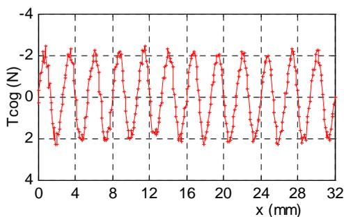
Fig. 14. Cogging force using the geometry of Fig. 11
