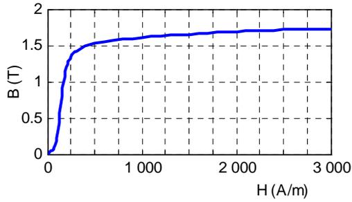
Fig. 6.  $B-H$  curve of the laminated sheet
