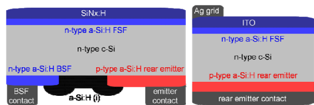
Figure 1 Sketches of the IBC Si-HJ (Left) and of the inverted Si-HJ (Right) cell.
