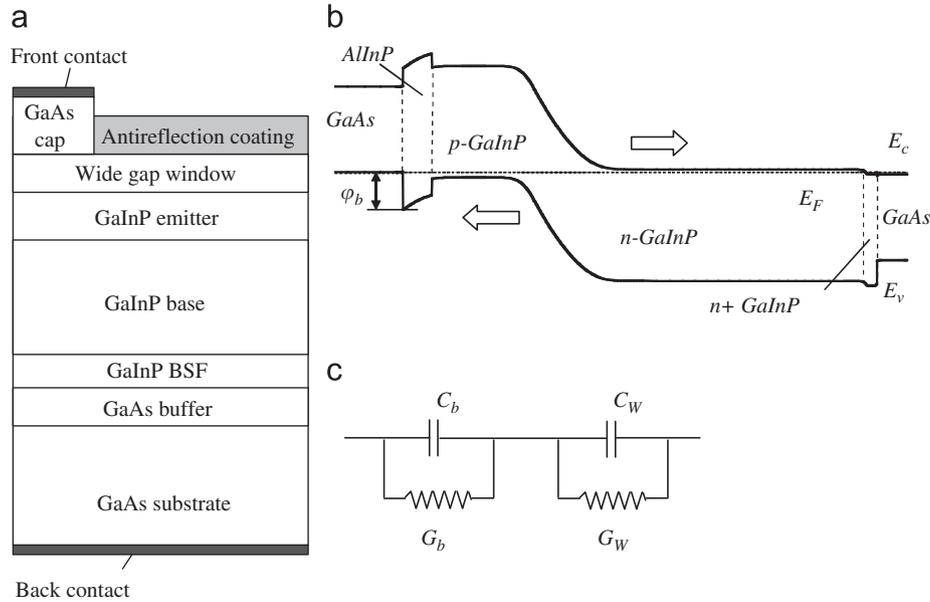
**Fig. 1.** Scheme of the GaInP solar cell (a). Schematic band diagram for p-n structure with p-AllnP window (b) and proposed equivalent circuit (c).
