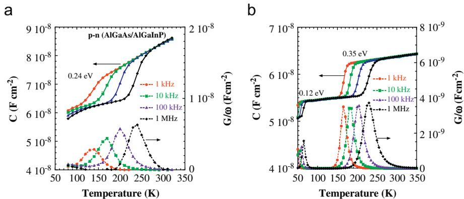
**Fig. 7.** Experimental  $C(T,f)$  and  $G/\omega(T,f)$  curves measured on p-n GaInP heterojunction with p-AlGaAs/p-AlGaInP window (a).  $C(T,f)$  and  $G/\omega(T,f)$  curves simulated with AFORS-HET 2.2 for the same structure (b).
