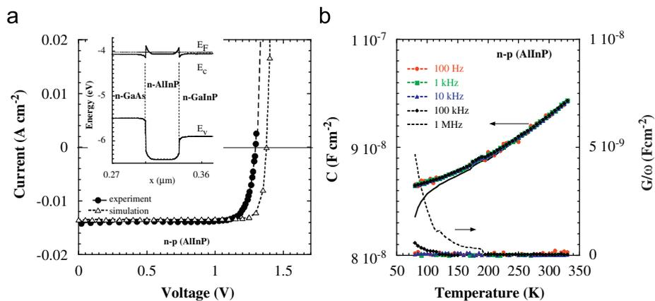
Fig. 5. Experimental and simulated  $I$ - $V$  curve of GaInP n-p solar cell with n-AlInP window under AM1.5 illumination (a). Calculated band diagram of the top interfaces is shown in the inset. Experimental  $C(T,f)$  and  $G/\omega(T,f)$  curves measured on the mesa structures (b).
