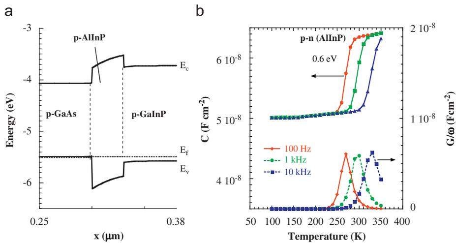
Fig. 4. Calculated band diagram of the top interfaces of GaInP p-n structure with p-AlInP window (a).  $C(T,f)$  and  $G/\omega(T,f)$  curves simulated with AFORS-HET 2.2 for the same structure (b).
