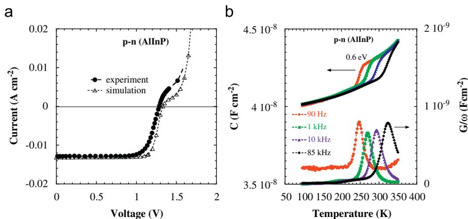
**Fig. 3.** Experimental and simulated *I*-*V* curve of GaInP p-n solar cell with p-AllnP window under AM1.5D illumination (a). Experimental  $C(T,f)$  and  $G/\omega(T,f)$  curves measured on the mesa structures, which were made on the same wafer (b).
