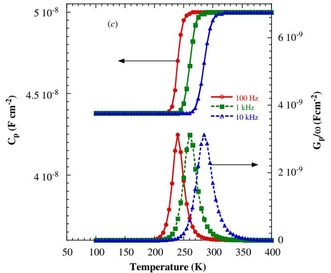
**Fig. 2.** Calculated curves of  $C_p$  and  $G_p/\omega$  versus temperature (C) for 100 Hz, 1 kHz and 10 kHz using  $C_w = 5 \times 10^{-8} \text{ F cm}^{-2}$ ,  $C_b = 3.5 \times 10^{-7} \text{ F cm}^{-2}$ ,  $G_0 = 10^9 \text{ } \Omega^{-1} \text{ cm}^{-2}$  and  $\phi_b = 0.6 \text{ eV}$ .
