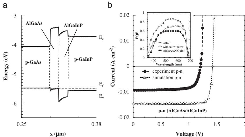
**Fig. 6.** Calculated band diagram of the top interfaces of GaInP p-n solar cell with p-AlGaAs/p-AlGaInP window (a). Experimental and simulated  $I$ - $V$  curve of this solar cell under AM1.5D illumination (b). The experimental external quantum efficiency for p-n solar cells with p-AlInP, without and with p-AlGaAs/p-AlGaInP window are presented in inset.
