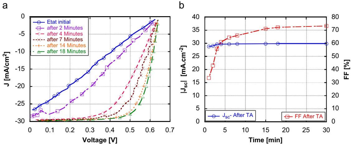
Fig. 2. AM 1.5 time dependent  $J(V)$  characteristics of (a) the same solar cell as in Fig. 1 (a) and time variation of the corresponding short-circuit  $J_{sc}$  current density and fill factor FF (b), after thermal air annealing at 200 °C, during 15 min.
