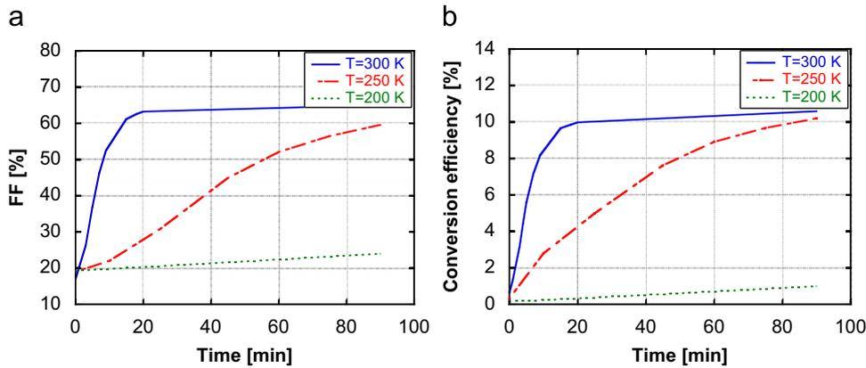
Fig. 3. Time variation under light soaking of the fill factor (a) and the conversion efficiency (b) of a non-annealed CIGSe/CBD-Zn(S,O,OH)/rf-ZnMgO/ZnO:Al solar cell, measured at AM 1.5 conditions for temperatures varying from 200 K up to room temperature.
