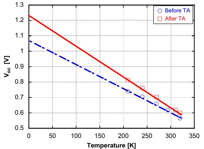
Fig. 5. Temperature dependence of the open-circuit voltage  $V_{oc}$  before and after thermal annealing at 200 °C.
