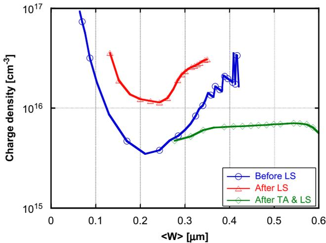
Fig. 4. Net charge density profile within the absorber of a CIGSe/CBD-Zn(S,O,OH)/rf-ZnMgO/ZnO:Al solar cell, measured for three states of the device, as explained in the text.
