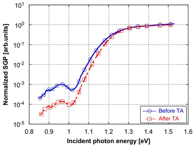
Fig. 6. Sub-gap photocurrent versus incident photon energy of solar cell before and after thermal air annealing.
