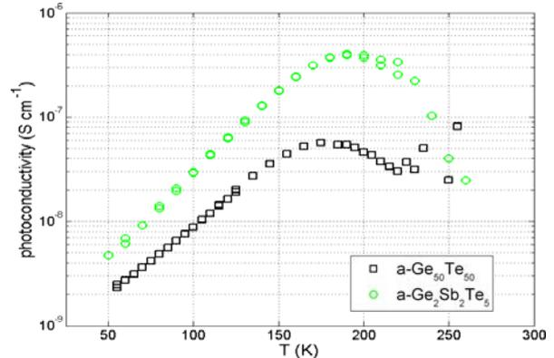
**Figure 3** Temperature dependence of the photoconductivity measured on 100 nm thick chalcogenide samples.
