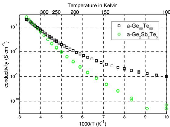
**Figure 1** Temperature dependence of the dark conductivity measured on a-Ge<sub>50</sub>Te<sub>50</sub> and a-Ge<sub>2</sub>Sb<sub>2</sub>Te<sub>5</sub> samples.
