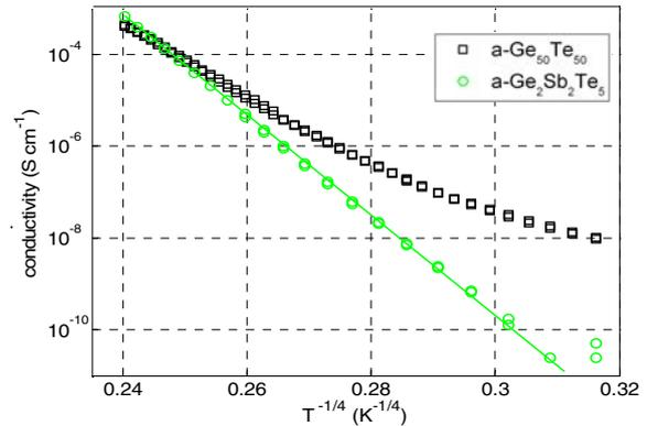
**Figure 2** Plot of the dark conductivity applying Mott law to the same data as in Fig 1 for both samples.
