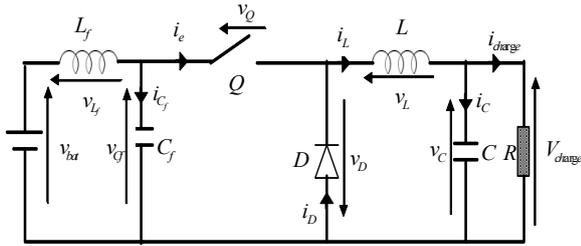
Fig. 6: Buck DC-DC converter
