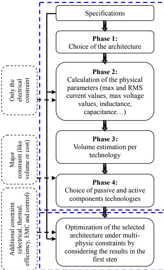
Fig. 1: Principle of the proposed pre-sizing approach
