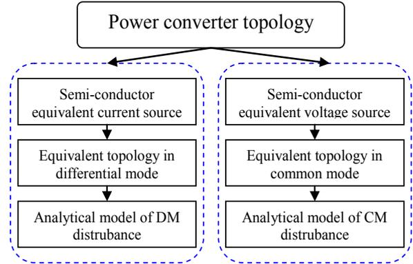
Fig 4 : Principle of the EMC model
