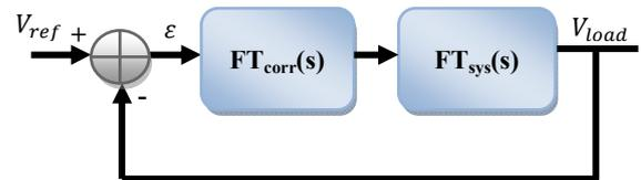
Fig. 8: closed control loop for the buck converter
