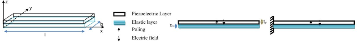
Figure 1: Geometric parameters for the piezoelectric unimorph actuator (3-D and side view) Free at both ends (left side view) and fixed-free (right side view) boundary conditions.
