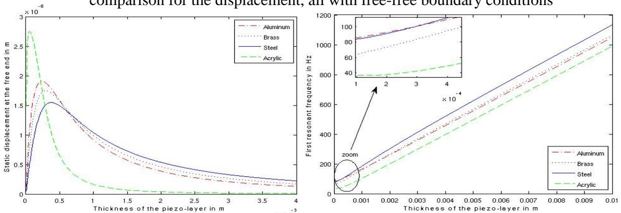
Figure 3: Displacement and first resonant frequency versus thickness of the piezo-layer for several elastic materials (obtained by the FE 1D model)
