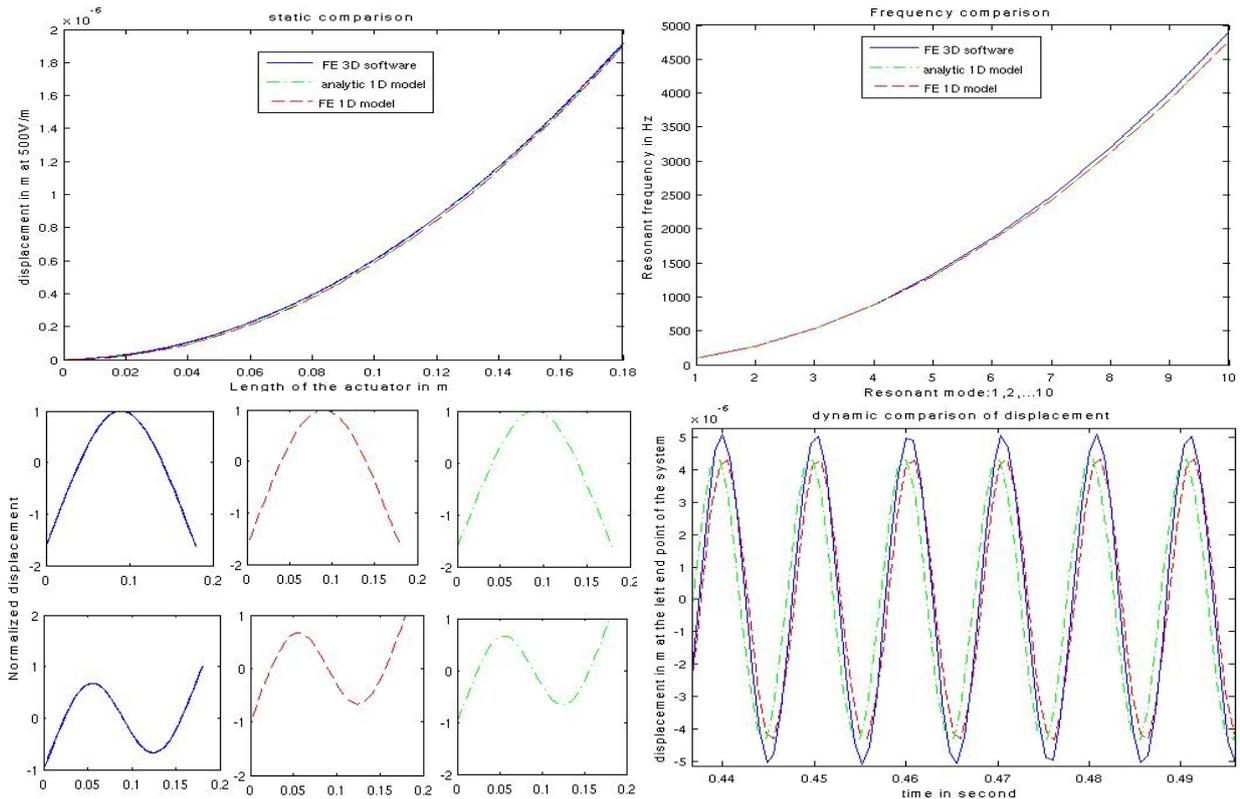
Figure 2: Static comparison for the tip deflection with fixed-free boundary conditions, frequency response for the 10<sup>th</sup> first mode, first and second mode shapes and dynamic comparison for the displacement, all with free-free boundary conditions
