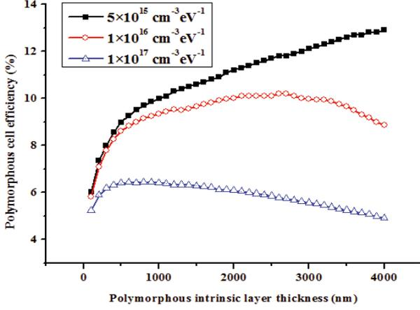
**Fig. 2.** Pm-Si:H cell efficiency as a function of pm-Si:H intrinsic layer thickness for three values of the Gaussian distribution peak value  $D_{\text{max}}$  (expressed in  $\text{cm}^{-3} \text{eV}^{-1}$ ):  $5 \times 10^{15}$  (■),  $1 \times 10^{16}$  (○) and  $1 \times 10^{17}$  (△).
