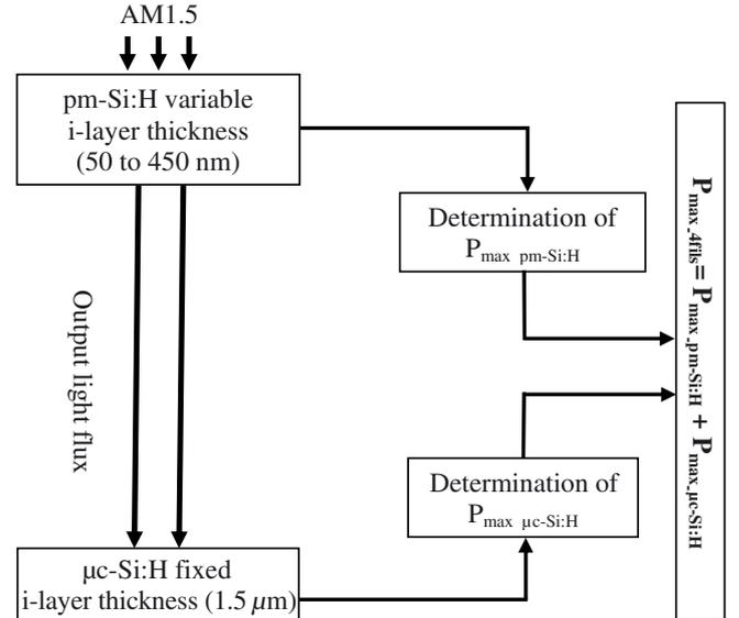
**Fig. 4.** Simulation steps for a four-wire tandem structure.
