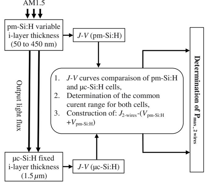
**Fig. 3.** Simulation steps for a two-wire tandem structure.
