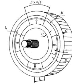
Fig. 3. The electromechanical actuator structure [13]
