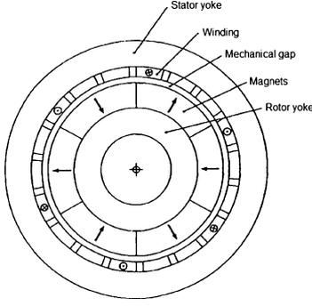
Fig. 3. Electromagnetic actuator structure.
