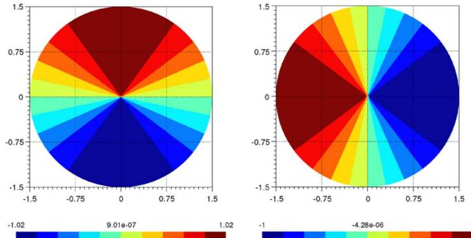
Fig. 4. Current density components at  $t = T/4$ : (left)  $J_x/J_c$ ; (right)  $J_y/J_c$ .
