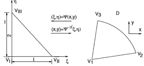
Fig. 1. Mapping of a triangle, from the (reference) parametric space to the physical space.
