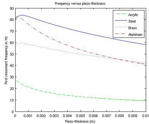
Fig. 4: Frequency versus piezo-thickness for different beam material
