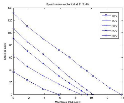
**Fig. 10:** Speed versus mechanical load for different applied voltage at 11.3 kHz.
