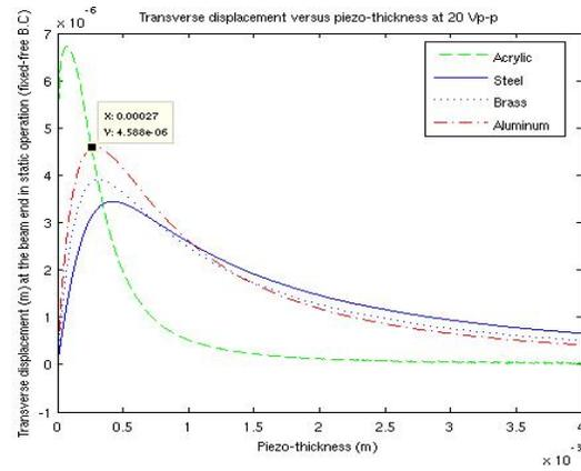
Fig. 3: Displacement versus piezo-thickness for different beam material
