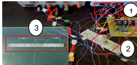
Fig. 5: Prototype (1: Signal generator, 2: power amplifiers and 3: robot body)
