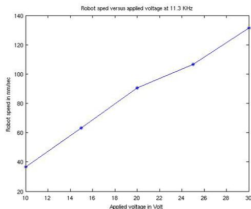
**Fig. 8:** Robot speed versus applied voltage on a smooth glass flat surface
