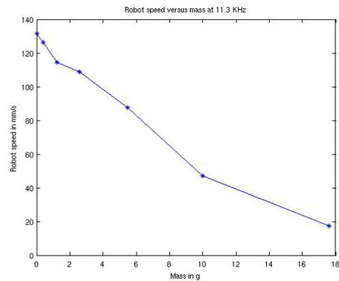
**Fig. 9:** Robot speed versus embedded mass on a smooth glass flat surface
