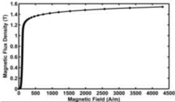
Fig. 11. B-H curve for M40050A metal sheets
