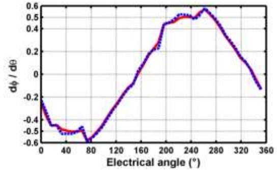
Fig. 13. Flux derivative under linear conditions at 150 A rated current .
