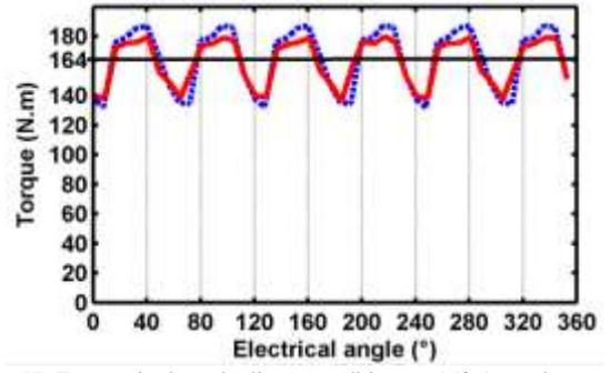
Fig. 17. Torque ripple under linear conditions at 150 A rated current. Dashed line-RelNet. Continuous line-2D.FEA
