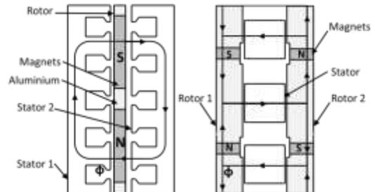
Fig. 19. On the left: Double stator/ single rotor IPM axial flux machine. On the right: Double rotor/ single stator IPM axial flux machine.
