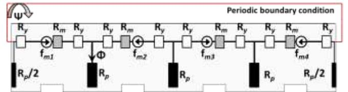
Fig.5. RelNet circuit for the rotor
