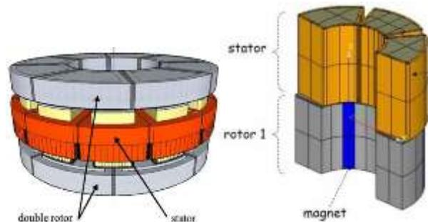
Fig. 1. Torus axial flux machine double rotor/single stator [8]
