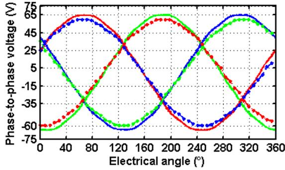
Fig. 20. Phase-to-Phase Voltage. Dotted lines-RelNet model. Continuous lines-Experimental results
