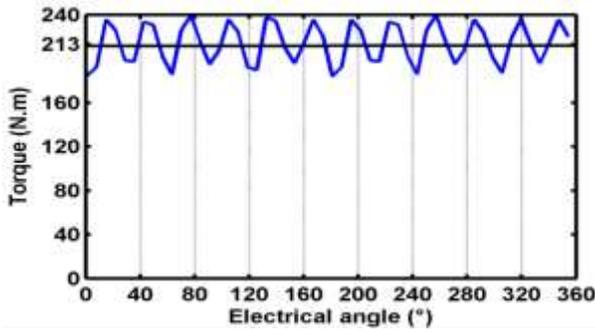
Fig. 21. RelNet torque ripple at 110 A rated current
