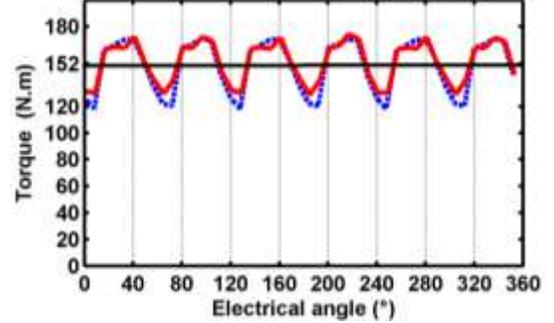
Fig. 18. Torque ripple under non linear conditions at 150 A rated current. Dashed line-RelNet. Continuous line-2D.FEA.
