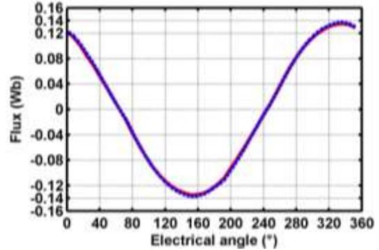
Fig. 12. Flux under linear conditions at 150 A rated current .
