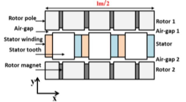
Fig. 4. 2D equivalent model of 2D 6-teeth 8-poles axial machine
