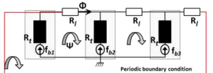
Fig. 6. RelNet circuit for half of the stator
