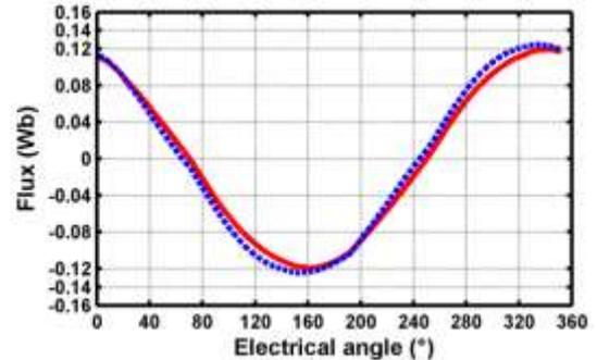
Fig. 14. Flux under non linear conditions at 150 A rated current .
