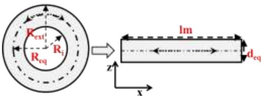
Fig. 3. 2D equivalent linearization
