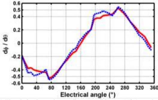
Fig. 15. Flux derivative under non linear conditions at 150 A rated current. Dashed line-RelNet. Continuous line-2D.FEA
