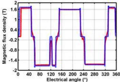
Fig. 16. No load normal flux density ( $B_n$ ) . Dashed line-RelNet. Continuous line-2D.FEA
