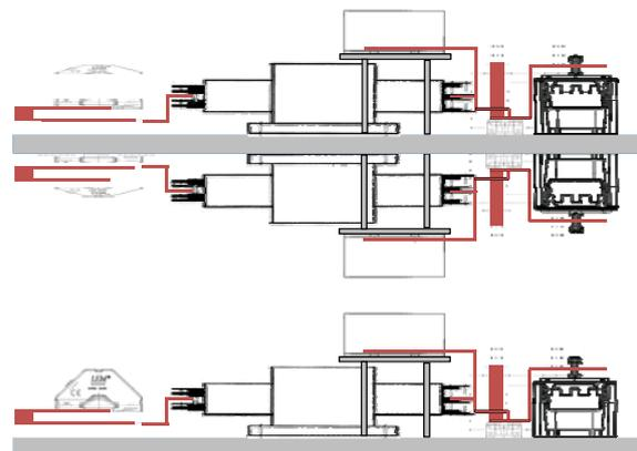
Figure 7b. Full 30kW converter implementation (symmetrical design over 2 heat-sinks)
