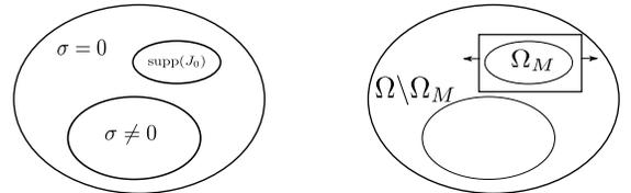
Figure 1: Domain  $\Omega$  for an EC case (left). Domain decomposition into a moving  $\Omega_M$  and a fixed  $\Omega \setminus \Omega_M$  subdomain (right).
