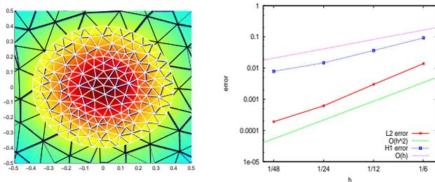
Figure 2: Focus on  $\Omega_M$  of the electric scalar potential and convergence rates in the fixed domain.
