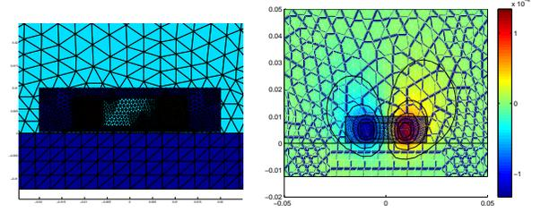
Figure 3: Focus on moving subdomain (left). Magnetic flux density (right).
