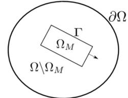
Fig.1: Domain decomposition between a moving subdomain  $\Omega_M$  and a fixed subdomain  $\Omega$ .
