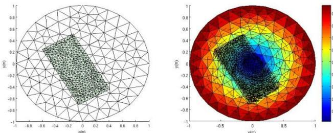
Fig.2:Overlapping meshes: fixed (coarse mesh) and moving (fine mesh) domains (left). Magnetic flux density (in  $\text{Wb}\backslash\text{m}^2$ )
