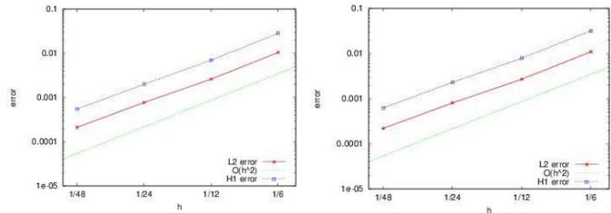
Fig.3: Convergence rates for the solutions in the fixed subdomain (left) and for the global solution (right).
